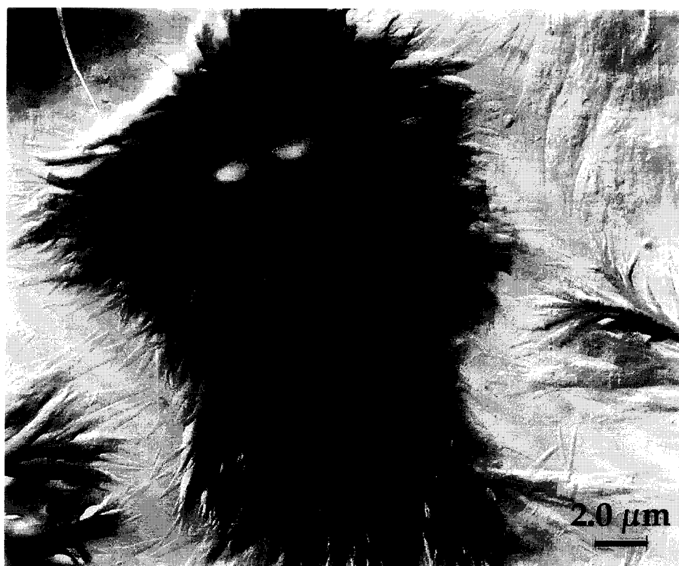
Figure 2 'Spherulitic' clustering of lamellae on their edges in PPOBC prepared by CTFMP (250°C, 4h)
